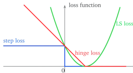
Figure 5: Step (0-1) loss, hinge loss, and squared loss. Squared loss is convex and differentiable, hinge loss is only convex, and step loss is neither.
